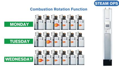
The controller automatically brings boilers on line, regulates outputs of other units, or switches off boilers as needed.
